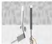
Clean the drill hole
